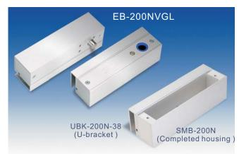
The unit may also be fitted semi-flush with the use of the SMB-200N completed housing. Or the EB-200N may also be fitted to a full glass door and glass frame application, using 2pcs of the SMB-200 Bracket and 2pcs of the UBK-200N-38 mounting brackets (EB-200NVGL). The thickness of glass are 14 mm maximum
